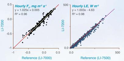
The figures to the left show hourly  $CO_2$  and  $H_2O$  fluxes measured with the LI-7200 Enclosed  $CO_2/H_2O$ Analyzer compared to fluxes measured with the LI-7000 and LI-7500 analyzers, which were used as standards. Fluxes measured with the LI-7200 were within 2.5% of the standards for all field experiments. These data were collected in 3 deployments that took place over four seasons. Data were collected over a ryegrass field and saw grass wetland.
